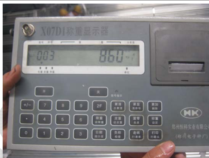
Product weight measurement (91pcs weight 860kg; equal distribution 1pc 9.45kg)
