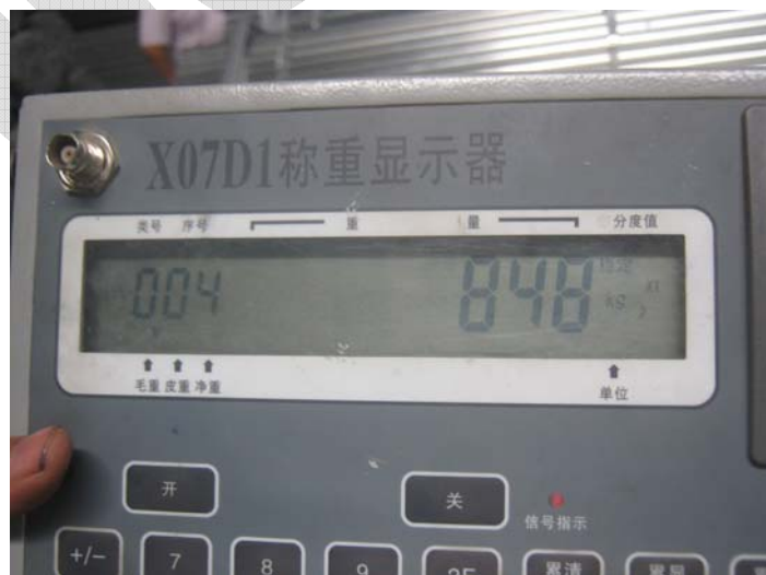
Product weight measurement (91pcsweight 848kg; equal distribution 1pc 9.31KG)
